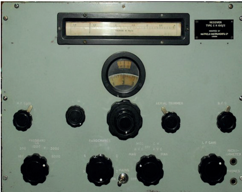
Figure 6: The Marconi CR-100 HF communications receiver used on the Pilot train and at Roberts Heights.
